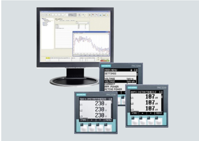
Components of the PC-based power management system
